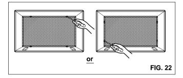
3 Ensure that the inside of the sleeve is thoroughly clean. Remove the backing from the Horizontal Insulation strip  $1_{3/8} \times 3_{/8} \times 27_{3/16}$  and attach that to the inside bottom of the sleeve as shown below. Remove the backing from the Around Insulation strip  $1_{3/8} \times 3_{/4} \times 61_{1/2}$  and attach that to the inside front of the sleeve as shown below.
